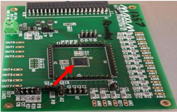
Fig. 2. Max 1257/1258 evaluation board
