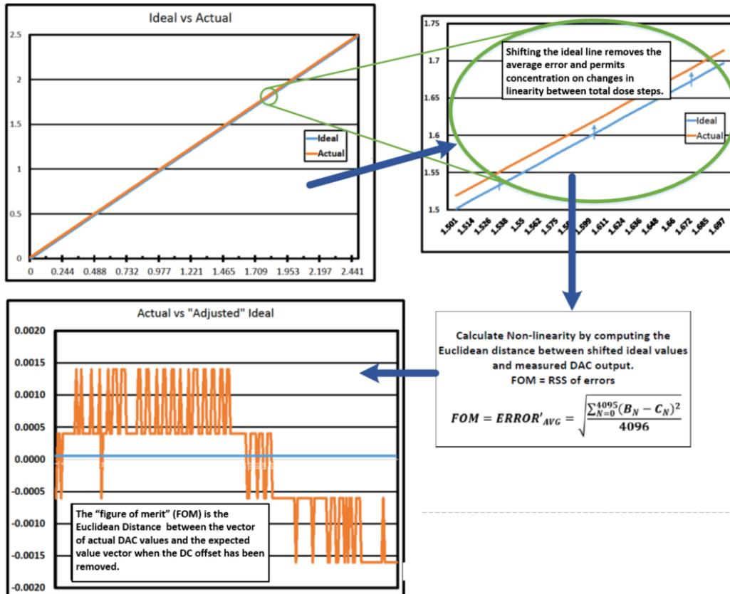
Figure 4. FOM calculation schematic
