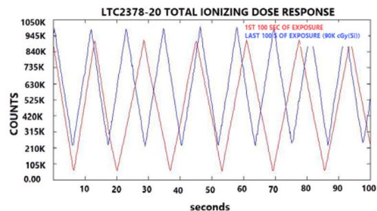
Figure 12. LTC2378 Conversion: 1<sup>ST</sup> 100 secs compared to last 100 secs
