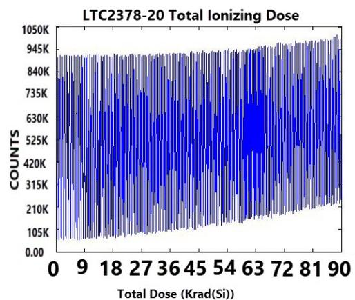
Figure 13. LTC2378-20 Conversion Over 90 Krad(Si) Exposure.
