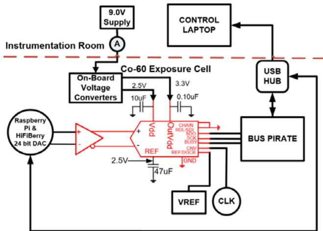
Figure 10. LTC2378-20 Configuration for total dose test
