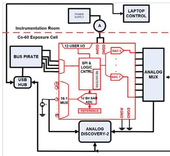
Figure 1. Max1257/1258 configuration for total dose testing
