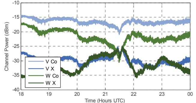
Fig. 4. Time series of received power levels during a snow event on December 26<sup>th</sup>, 2015 showing strong depolarization effects during the height of the event at approximately 21:30 UTC.
