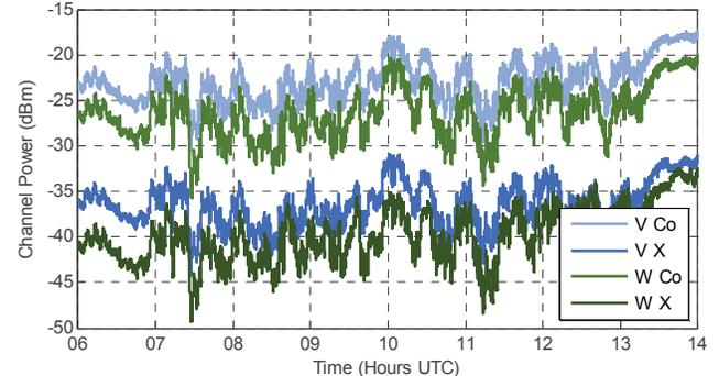
Fig. 5. Time series of received power levels during a cloud event on January 9<sup>th</sup>, 2016. From approximately 07:00 – 13:15 UTC, clouds passed along the link introducing variations in attenuation up to 15 dB.
