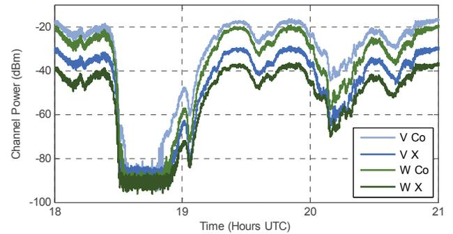
Fig. 3. Time series of received power during a deep rain fade on November 4<sup>th</sup>, 2015. Total attenuation exceeds the receiver dynamic range on all channels for approximately 24 minutes from 18:31 - 18:55 UTC.
