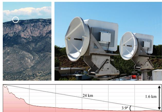
Fig. 1. The location of the transmitter atop Sandia Crest (left); the V and W-band receivers in Albuquerque, NM (right); and the elevation profile of the slant path covered by the link (bottom).
