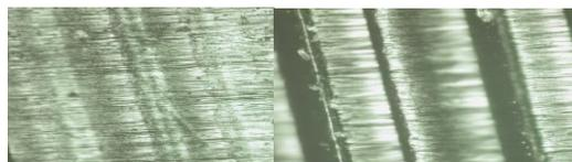
Fig. 4 Printed substrate before (left) and after (right) Sr-90 exposure illustrating the manifestation of defects where top picture shows between printed layers and bottom shows face of a single layer with increasing defects.
