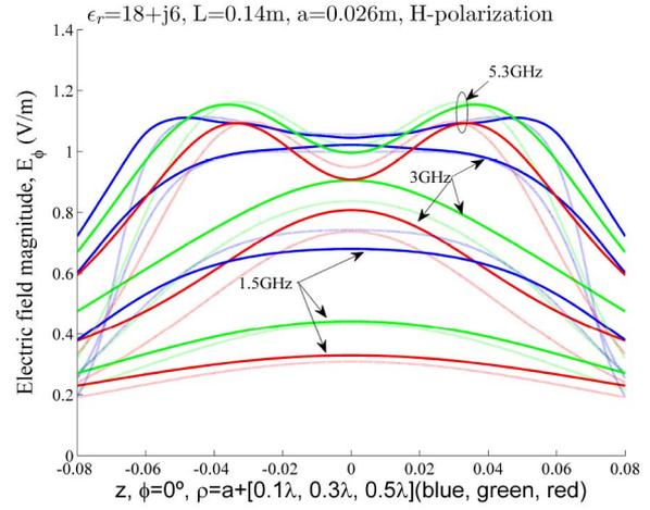
Fig. 5. Scattered electric field magnitude in the near field for cylinder 3. (Dark lines) MM method. (Light lines) Proposed approximation of this letter.
