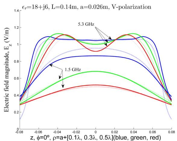
Fig. 6. Scattered electric field magnitude in the near field for cylinder 3. (Dark lines) MM method. (Light lines) Proposed approximation of this letter.
