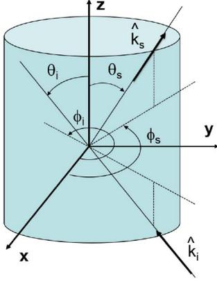
Fig. 1. Cylinder reference system.
