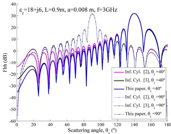
Fig. 8. HH bistatic scattered coefficient.
