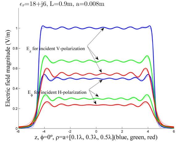
Fig. 2. Scattered electric field magnitude in the near field for cylinder 1. (Dark lines) MM method. (Light lines) Proposed approximation of this letter.
