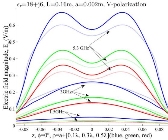
Fig. 4. Scattered electric field magnitude in the near field for cylinder 2. (Dark lines) MM method. (Light lines) Proposed approximation of this letter.
