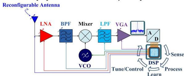
Fig. 2. Block diagram of the proposed reconfigurable receiver
