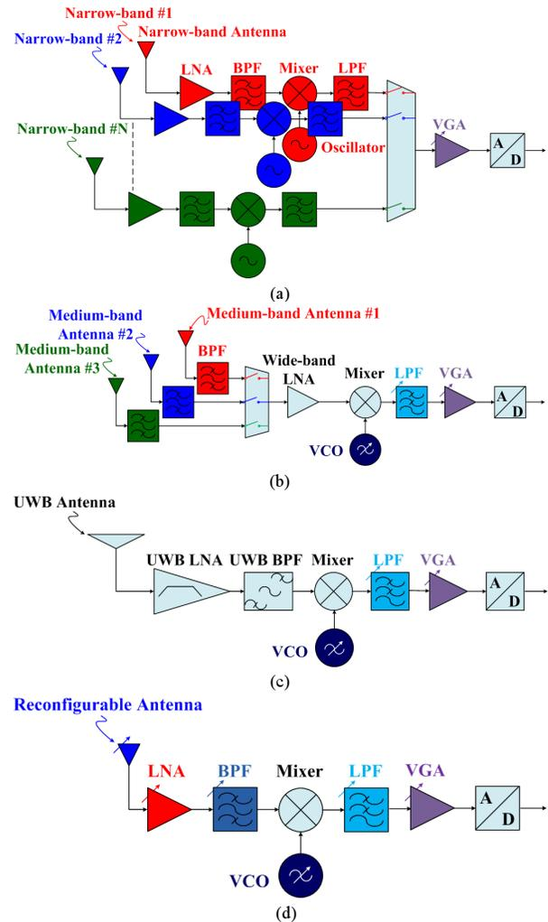
Fig. 1. RF front-end architecture: (a) multiple narrow-bands, (b) wide-band with few medium bands, (c) ultra-wideband, and (d) reconfigurable
