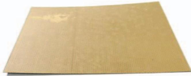
Fig. 2. Carbon epoxy layup layered with phosphor bronze mesh
